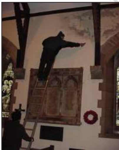
Taking Gann meter readings
