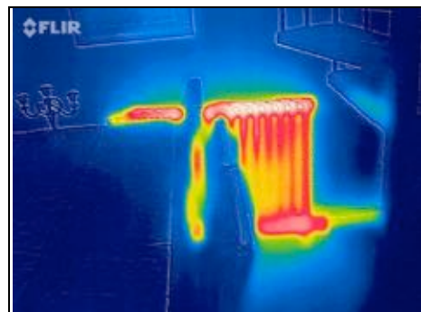
Thermal image photograph – the red showing heat loss from radiator
